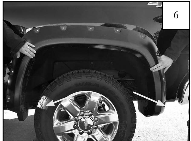
Loosely attach flare with factory screws removed previously.
